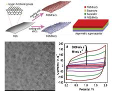
Hematite quantum-dot/functionalized graphene-sheet composites are prepared and the composite electrode can reach a maximum specific capacitance of 347 F g $^{-1}$ , which is much larger than the reported values for the Fe $_2$ O $_3$ -based electrodes in neutral aqueous electrolyte. A high-performance 2 V asymmetrical supercapacitor is fabricated using Fe $_2$ O $_3$ /FGS as anode and MnO $_2$ /FGS as cathode in 1 M Na $_2$ SO $_4$  electrolyte.
