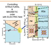
Rare-earth substituted BiFeO<sub>3</sub> (BFO) holds great promise as a piezoelectric and magnetoelectric material. A firstprinciples based scheme is developed to investigate the structural and magnetic transitions of Nd-doped BFO at finite temperatures. Thanks to this new method, the nature of the compositioninduced transformations is unveiled, and the possibility to control the magnetic order by an applied electric field is demonstrated.
